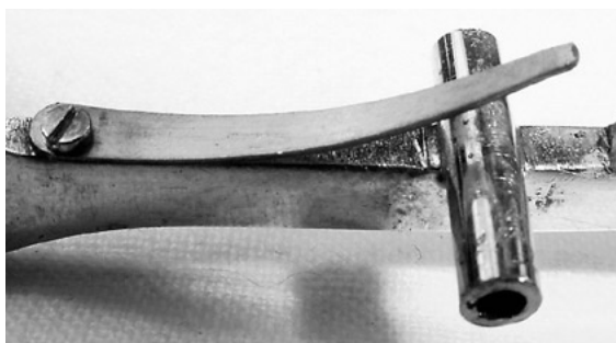
Flat spring screws may become loose
