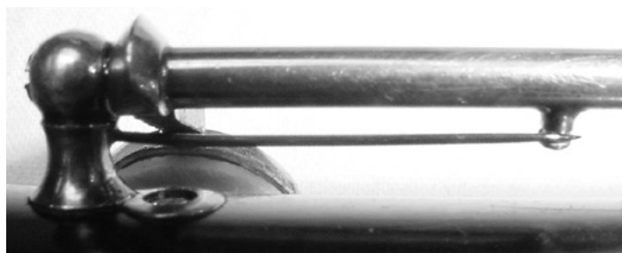
Round spring hooks into the spring cradle
