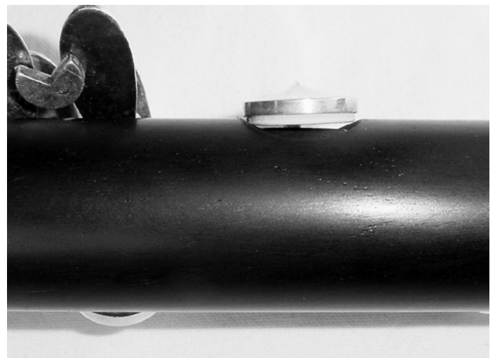
Pad cup is not parallel to the tone hole face
