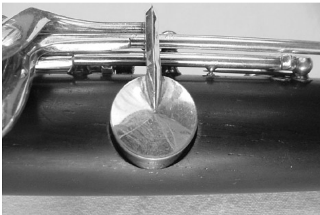
Pad cup is centered over the tone hole
