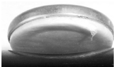
Tears in the bladder skin may cause leaks
